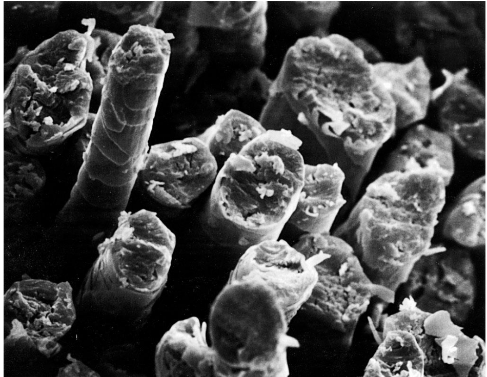
Magnified wool fibers have the appearance of scaly worms. Courtesy, American Wool Council
